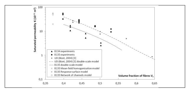
Figure 1: Comparison of the different methods for determination of longitudinal warp permeability in saturated regime.
